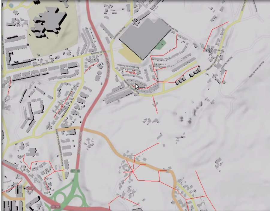
Figure 5.9: Aerial cables are represented as red lines. The 3D buildings, the aerial cables and the OSM texture fit together perfectly.
