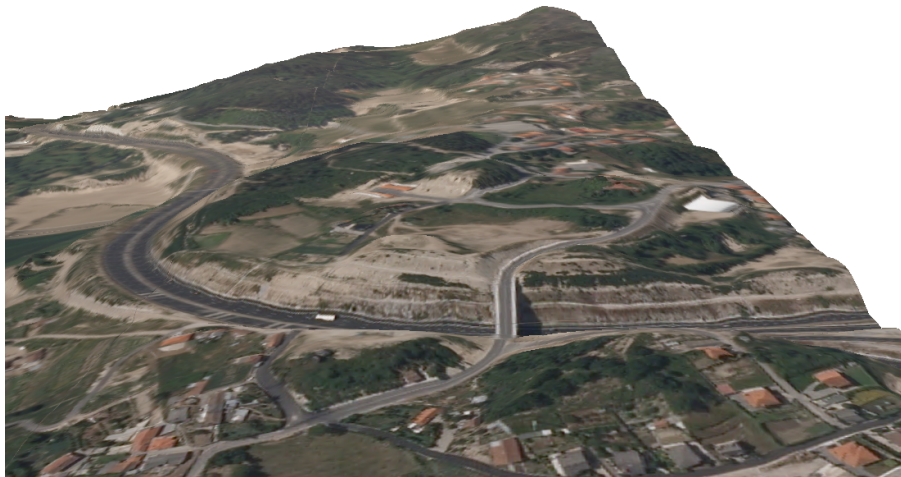
Figure 5.7: Tile obtained using W3DS GetTile operation. The aerial image texture is obtained from a WMS server.
