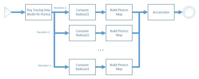
Figure 4.12: Fluxogram of PPMPA with concurrent iterations
