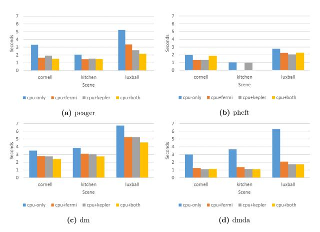
Figure 6.6: Avg. iteration time of the different schedulers with GPU devices
