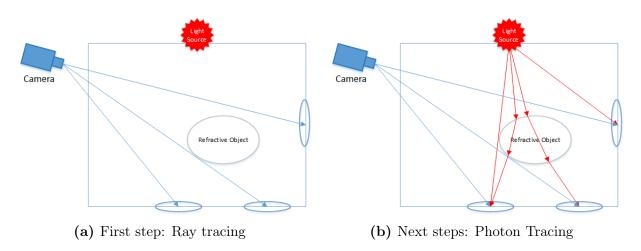
Figure 4.8: Overview of Progressive Photon Mapping
