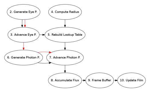
Figure 5.2: Dependency graph of an iteration of SPPMPA. Red arrows represent dependencies related to the seed buffer, which are not imposed on the algorithm itself, but only a limitation of the implementation
