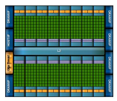
Figure 2.1: Overview of the Fermi Architecture (from NVidia documentation)
