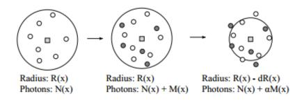
Figure 4.9: Radius Reduction after a Photon Tracing step
