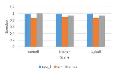
Figure 6.5: StarPU implementation, CPU sequential vs sequential schedulers
