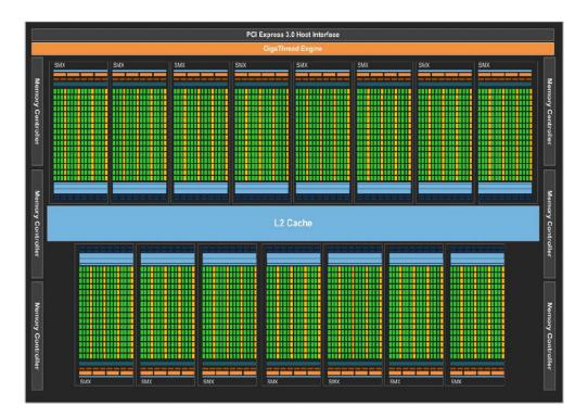
Figure 2.2: Overview of the Kepler Architecture (from NVidia documentation)
