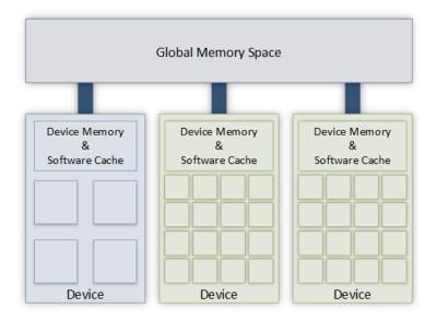
Figure 3.1: GAMA memory model, an extension to the one shown in Figure 2.4
