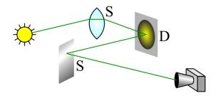
Figure 4.5: Specular to Diffuse to Specular path (SDS)
