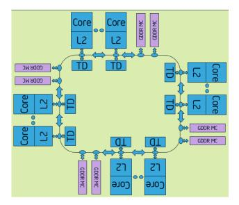
Figure 2.3: Overview of the MIC Architecture (from www.theregister.co.uk)
