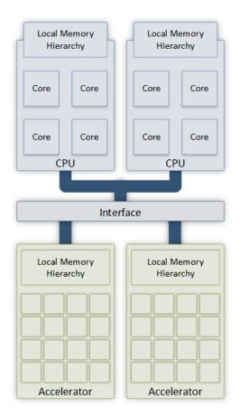
Figure 2.4: Example diagram of a HetPlat
