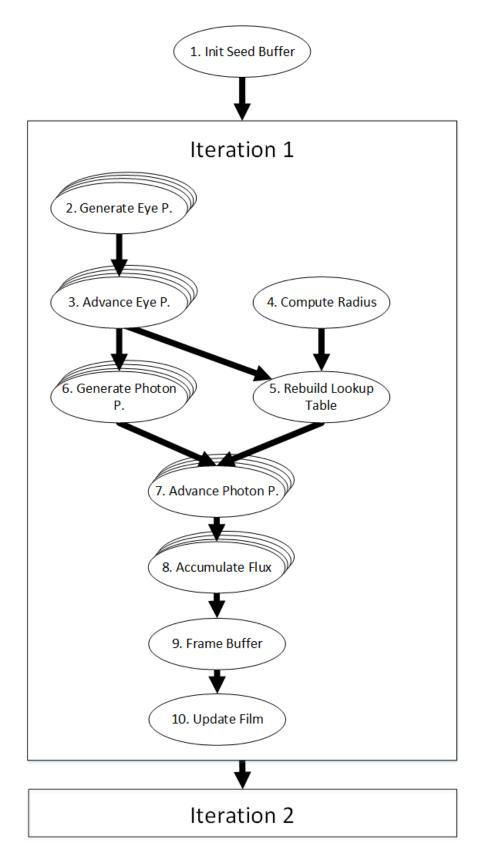
Figure 5.1: Diagram of the SPPMPA computational tasks and execution order. Tasks 2, 3, 6, 7, 8 can be parallelized. All other are sequential. The SPPMPA algorithm actually allows independent iterations, which is not represented in this diagram.
