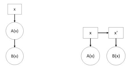
(a) A and B are executed in order, and the same(b) A and B are scheduled to different devices, buffer for x is re-used creating a temporary copy of x
