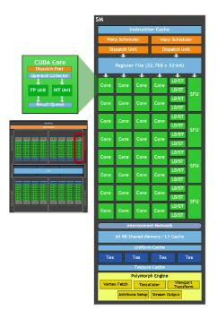
Figure 2.7: Fermi Architecture. - Fermi architecture (35).
