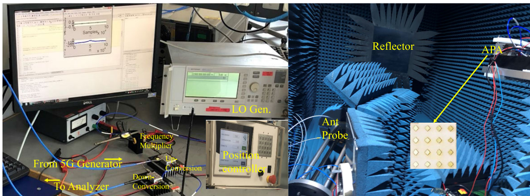
FIGURE 4. Measurement setup using compact antenna test range chamber.
