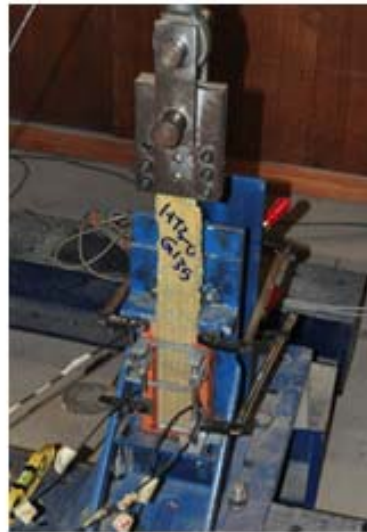
Figure 6: Single-lap shear bond test setup.
