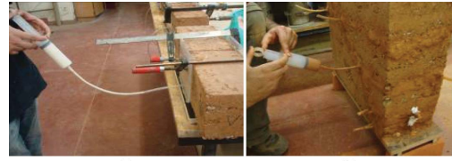
Figure 7. Injection of the (a) beam-specimens and (b) wallet-specimens. (Credits: Authors).
