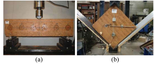
Figure 5. Tests carried out on the rammed earth specimens: (a) three-point bending and (b) diagonal-compression. (Credits: Authors).
