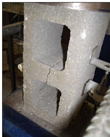
Figure 8: Behaviour of 2C-units under compression parallel to bed joints.
