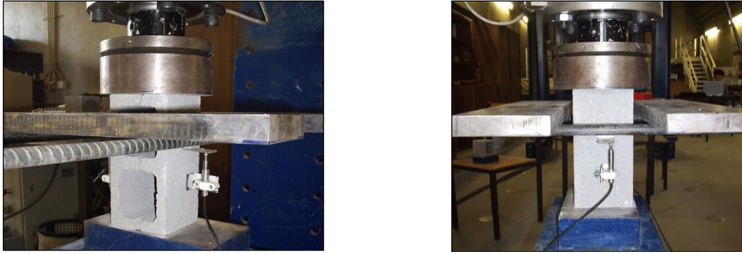
Figure 5: Test setup of the compressive tests in direction parallel to bed joints.
