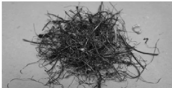
Figure 2. Recycled steel fibers extracted from rubber tires
