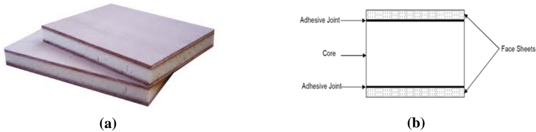
Figure 1. a) Type of sandwich panel; b) Details of sandwich panel [2]
