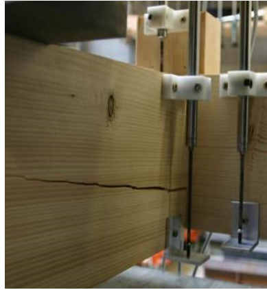
Fig. 2: Failed test specimen
