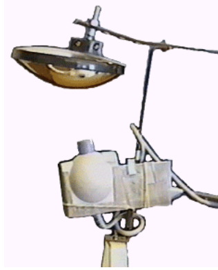
Figure 2: Figure 2: Mirror and Camera Support (side view)
