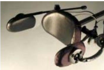
Figure 2 Head array controller, from Adaptive Switch Lab. Inc
