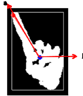
Figure 8 Vectors used in the calculation of finger orientation
