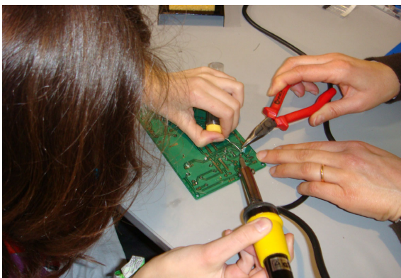
Figure 2. Soldering the components to build the robot
