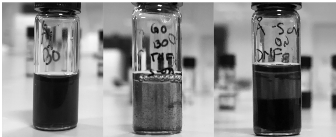
Figure 5.4: Asphaltene, GO, and both asphaltene + GO dispersed in saturates + DBSA.
