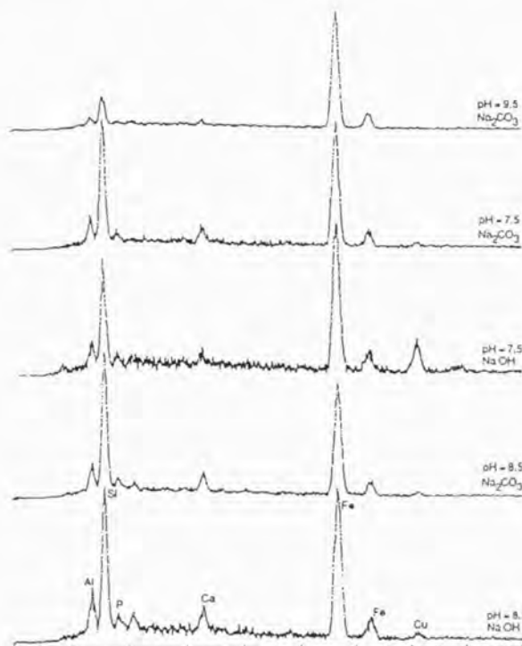
Figure 6 - Qualitative analysis of the deposits of magnetite particles on copper tubes obtained by EDS.
