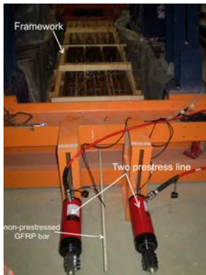
Figure 2: Prestressing system using a coupler hydraulic jack
