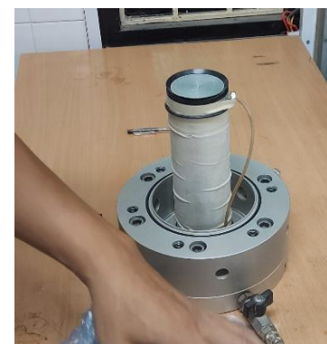
(c) Put the sample into the cyclic triaxial compression chamber
