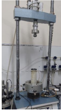
(a) Install the sample into the cyclic triaxial compressor
