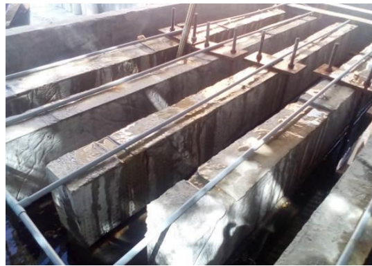
Fig. 2 – Seawater spraying system on testing beams.
