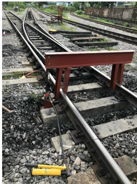
Fig. 3 – Measuring railway bed stiffness at the site of turnout
