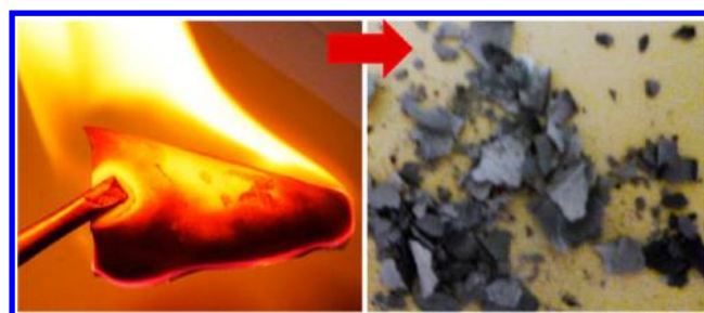
Figure 7. Representative image showing the possibility to incinerate the SH paper substrates up to an ash residue.
