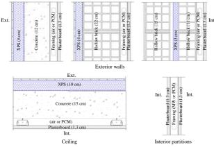
Figure 3 Composition of walls and roof.
