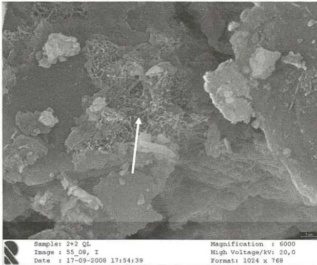
Fig.4 SEM of chitosan (3%) and latex (1%) – presence of C-S-H gel [18].
