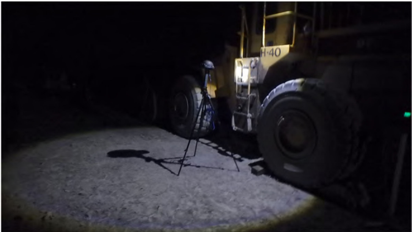
Fig. 3. Area luminaire-1 pattern displayed in setup for measurements associated with ingress/egress on the CAT 980C wheel loader
