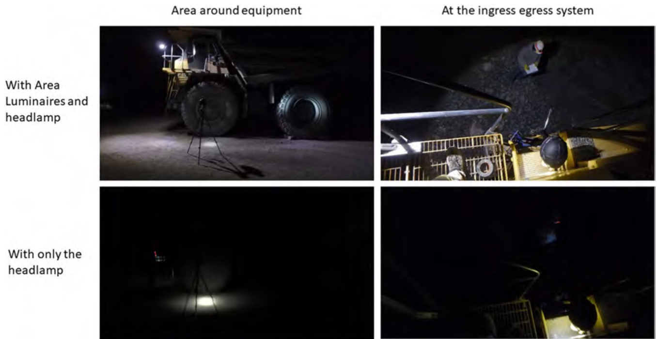
Fig. 13. Comparison of the area illuminated using the LED area lighting plus the headlamp (top left and right images) versus the headlamp only (bottom left and right images). The scenes depicted are at ground level on the driver’s side of the equipment (left images) and at the top platform of the ingress/egress system (right images)
