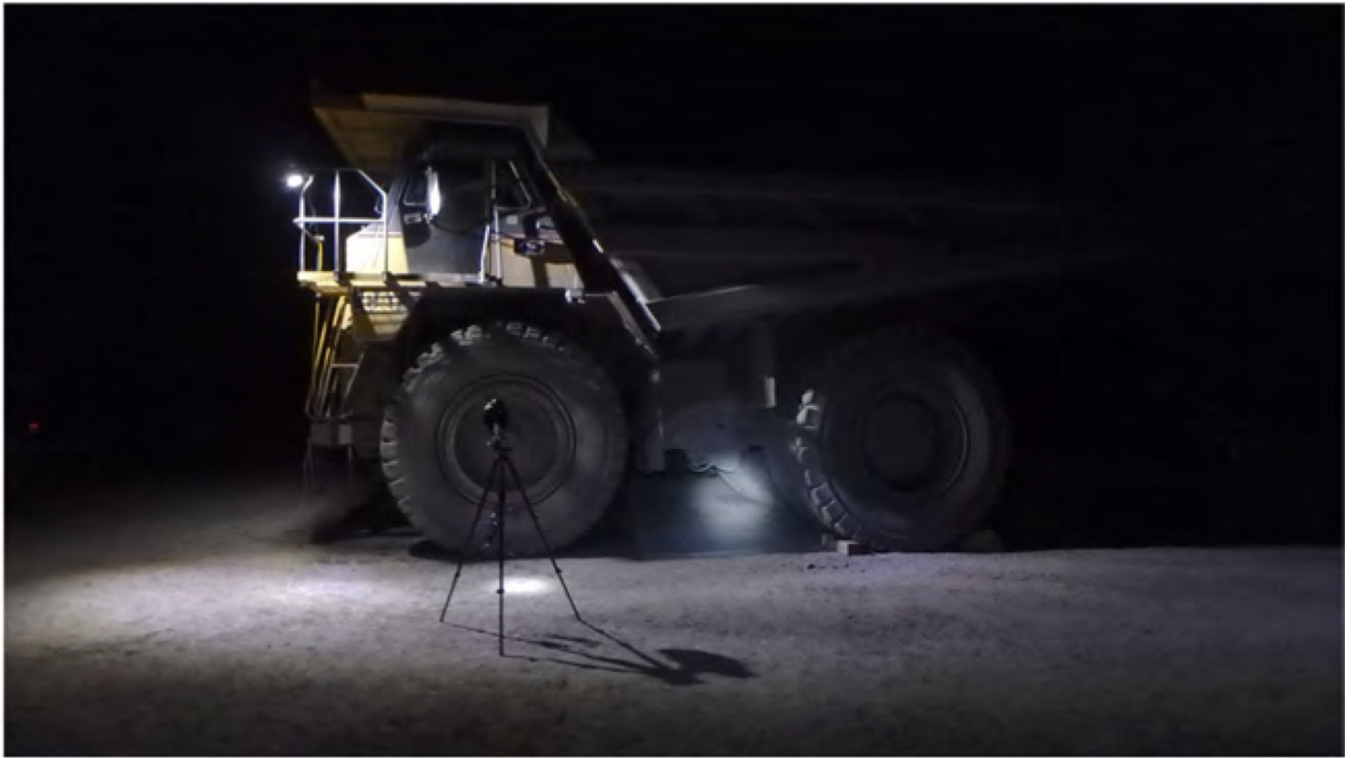
Fig. 4. Area luminaire-2 beam pattern displayed in setup for measurements associated with the pre-shift walkaround tasks on the Komatsu HD785 haul truck
