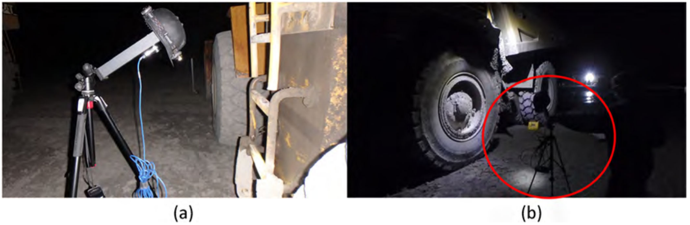
Fig. 5. The setup for measurements that represent a mine worker at (a) the ladder (first rung) of the smaller front-end loader and (b) the ground at the driver's side front tire of the haul truck during pre-shift walk-around
