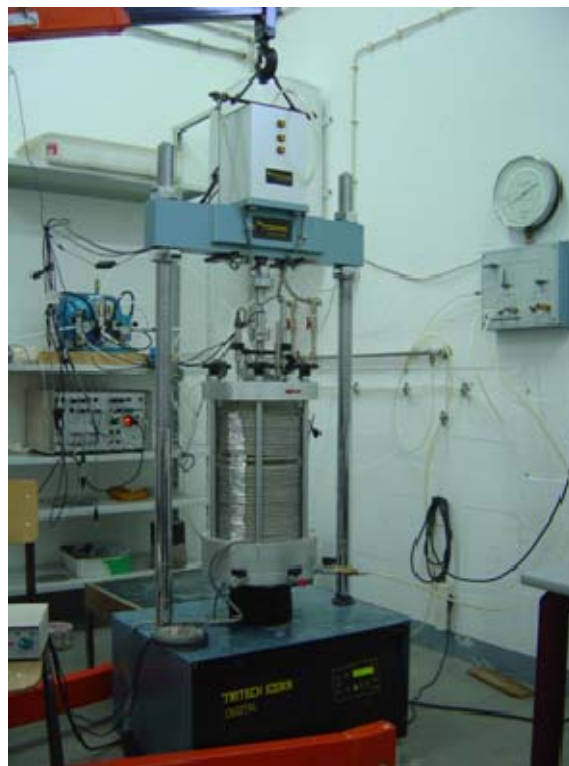
Figure 5. Triaxial equipment of Lab of Road Pavement Mechanics of the Department of Civil Engineering of the University of Coimbra
