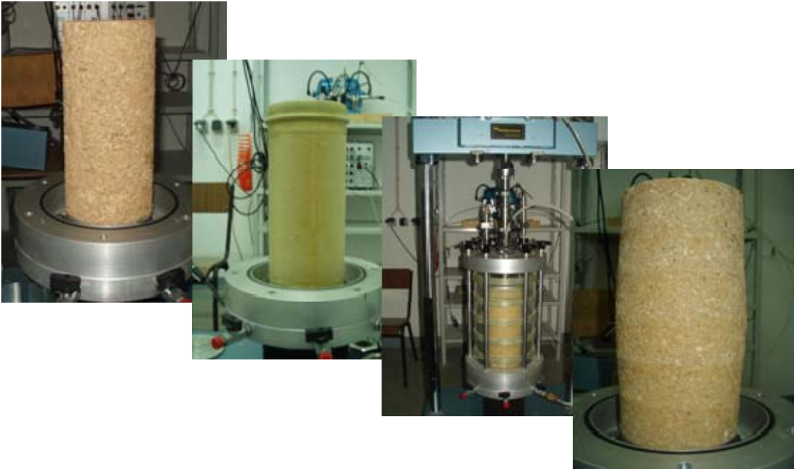
Figure 6. Limestone specimen: after compaction, with the membrane, in the camera during the test and after the test
