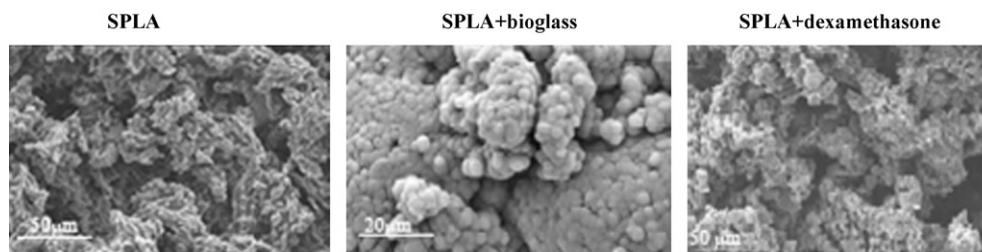
Fig. 6. SPLA-based matrices prepared by supercritical assisted phase inversion.
