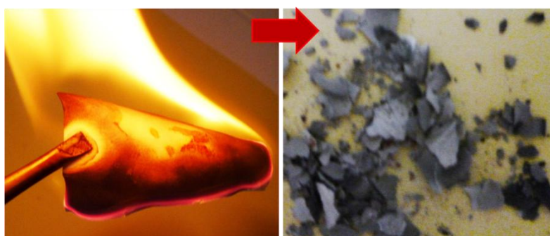
Figure IV. 7 - Representative image showing the possibility to incinerate the SH paper substrates up to an ash residue.
