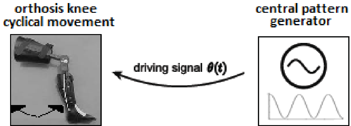
Figure 5.1: Sketch of the swinging task. The CPG generates the rhythmic signal to the controlled joint.
