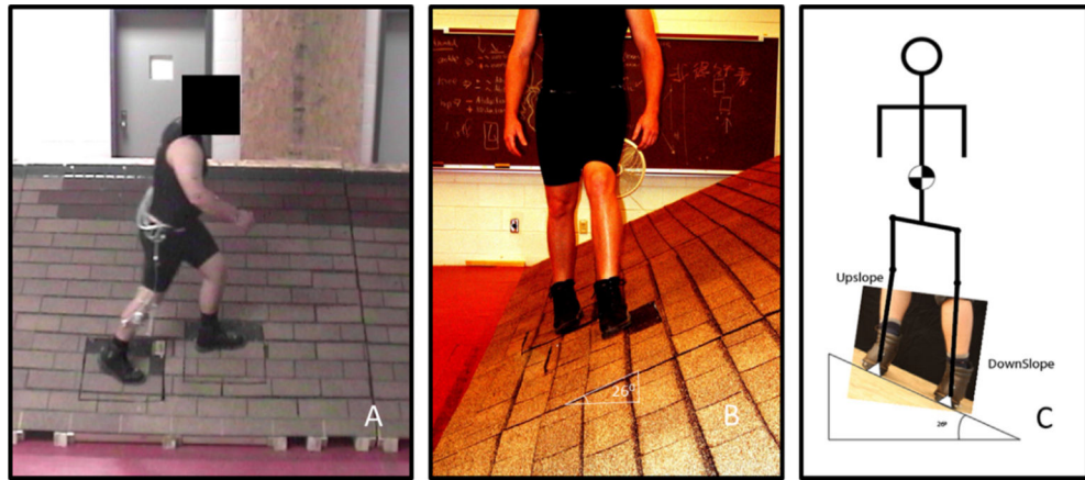
Fig. 1. (A) Sagittal view of subject traversing the roof segment. (B) Frontal plane anterior view of subject traversing the roof segment. (C) A posterior frontal plane rendering of a subject traversing across the 26° roof surface. The left foot was the upslope foot and right was downslope.
