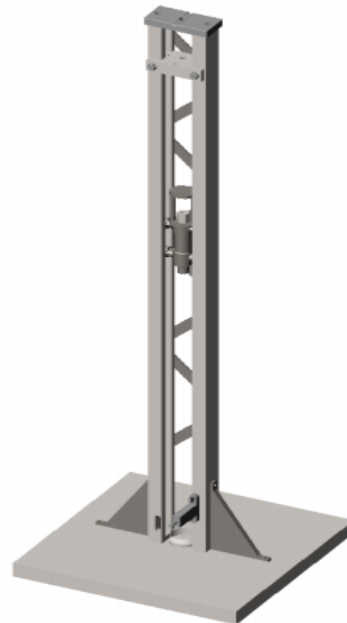
Fig. 1 Drop tower designed for dynamic impact in cartilage tissue
