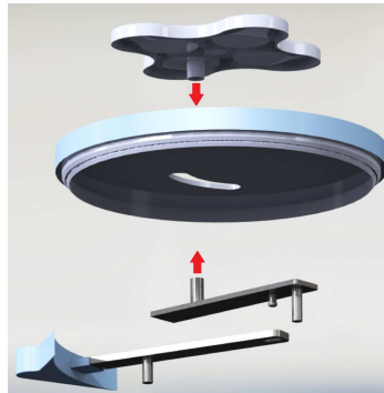
Figure 6: Mechanical restriction for coupling the plates with other parts of the mechanical system.
