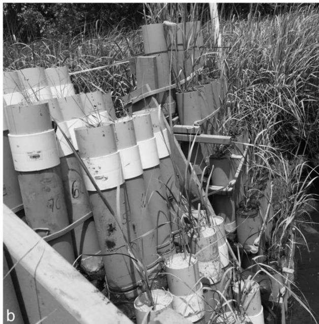
Figure 2. (A) Setup of three marsh organ structures placed side by side in a tidal creek. Brackets on the left show elevation ranges of habitat types of the adjacent marsh. Letters indicate pot treatments: SP C = S. patens controls, SP TLP = S. patens thin-layer placement, SA C = S. alterniflora controls, SA TLP = S. alterniflora thin-layer placement. (B) Experimental pots after 10 cm of sand was added to TLP treatments.
