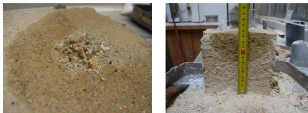
Figure 18 – Pitting depth and depth of moisture penetration.
