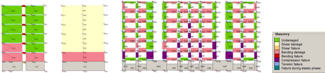
Figure 13. Damage in the walls in "+Y" direction at the failure stage: (a) W-Y4; (b) W-Y6; (c) W-X1; (d) legend.
