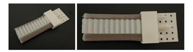
Figure 63. Attached granular jamming component filled with granular material (Ground Coffee)
