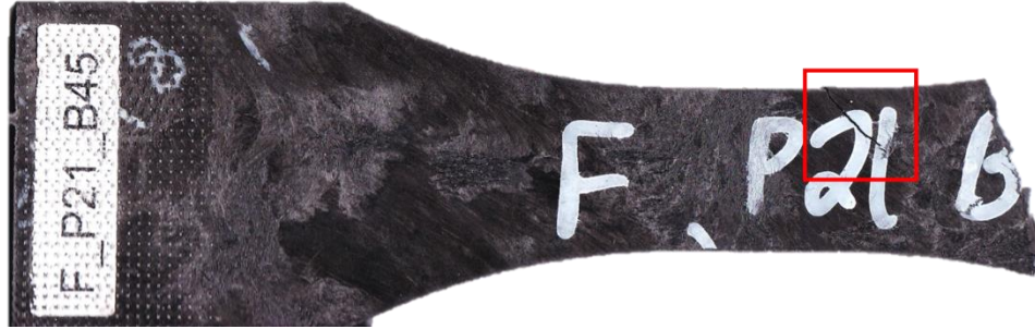
Figure 4.20: 45° fatigue sample P21B45 loaded to a peak stress of 83 MPa, arrested fatigue crack propagation
