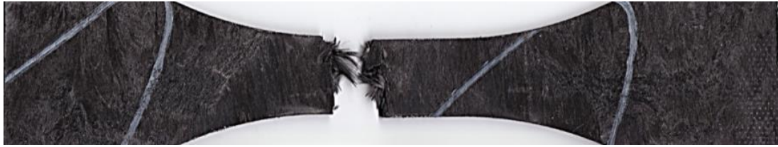
Figure 4.27: 90° specimen P18A90, failure after 34 cycles with a peak stress of 48 MPa
