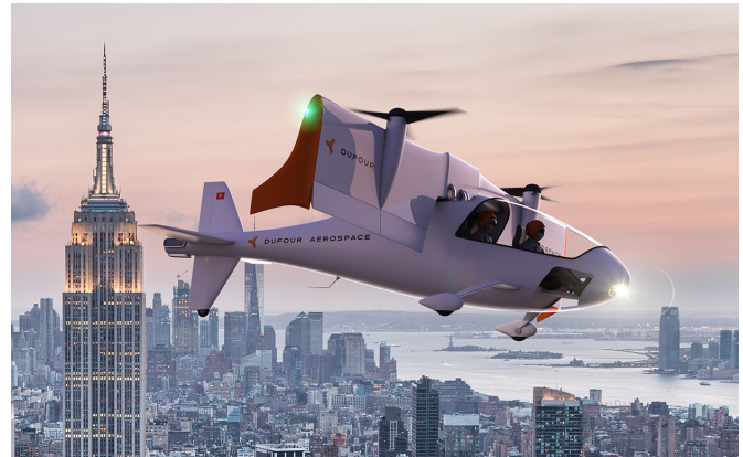
Fig. 1. A rendering picture of the Dufour Aerospace aEro2 Tilt-Wing Aircraft in helicopter mode
