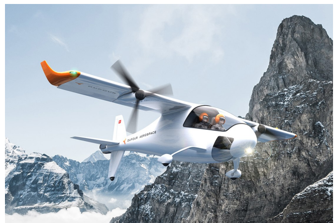
Fig. 2. A rendering picture of the Dufour Aerospace aEro2 Tilt-Wing Aircraft in airplane mode
