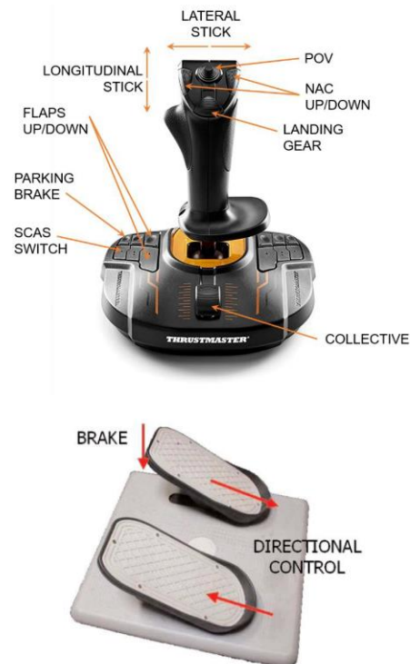
Figure 5: the hardware adopted in the tilt-rotor flight simulation platform. Top panel, the flight stick. Bottom panel, the rudder pedal.
