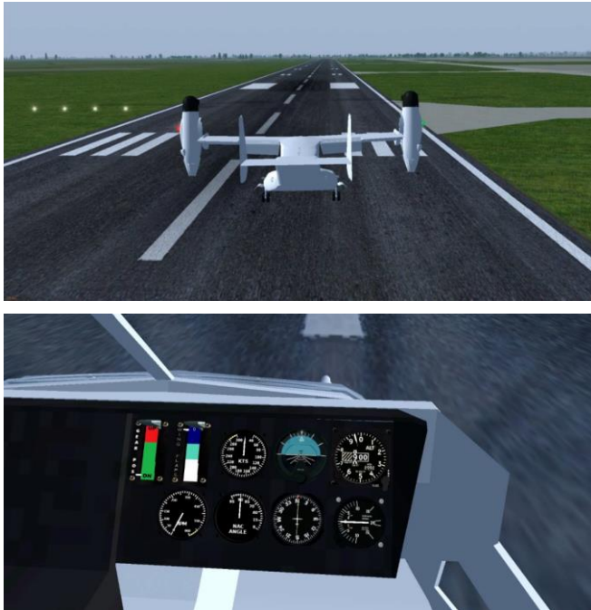
Figure 4: screens captured from FlightGear simulator. Top panel, the aircraft in the simulated environment visualized with the external view. Bottom panel, the Primary Flight Display implemented to interact with the pilot.
