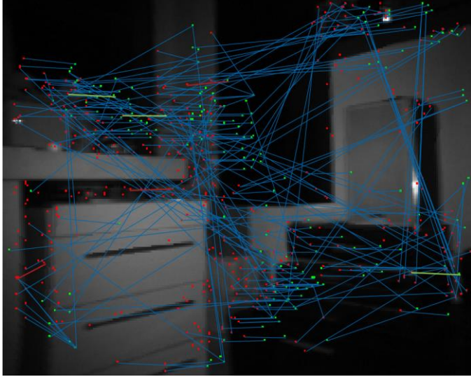
Fig. 1. Sample B/W-Image with drawn feature points, part of a sequence in which the camera got rotated. Green dots: Frame k-1 Red dots: Frame k Lines: Brute-Force matches
