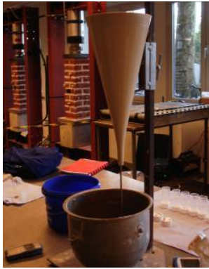
Fig. 4 – Marsh's cone used in the tests (dimensions in mm).
