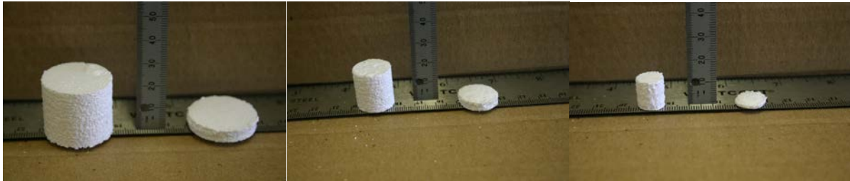
Figure 2: Test samples before and after quasi-static testing (large [L], medium [C], small [R])
