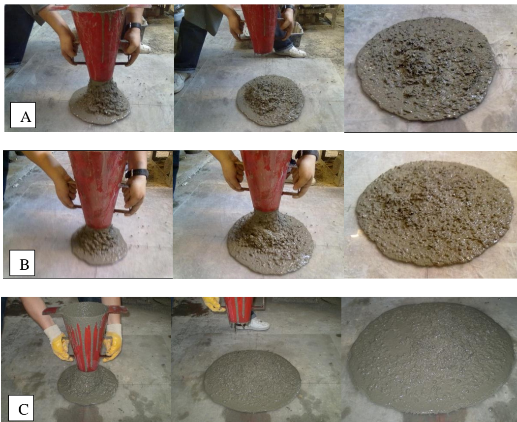
Fig.22 Slump flow of SCC contains 47% (A), 48% (B) and 48.6% (C) past
