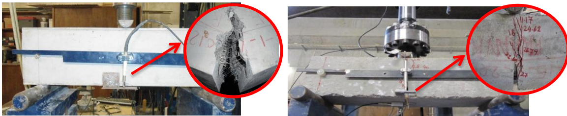
Fig.24 Three-point bending test with the notch (left) 25mm and (right) 60mm high
