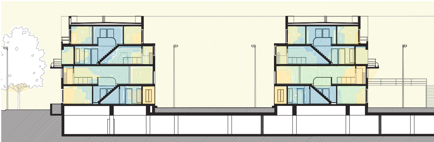
Figure 5.3.4.3. Section showing the amount of natural light entering the building (Simulation results of variation4).
