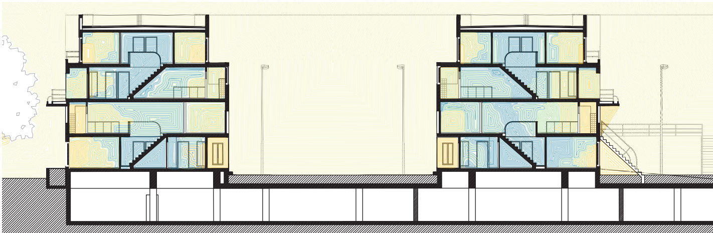
Figure 5.3.3. Section showing the amount of natural light entering the building (Simulation results of the existing building).
