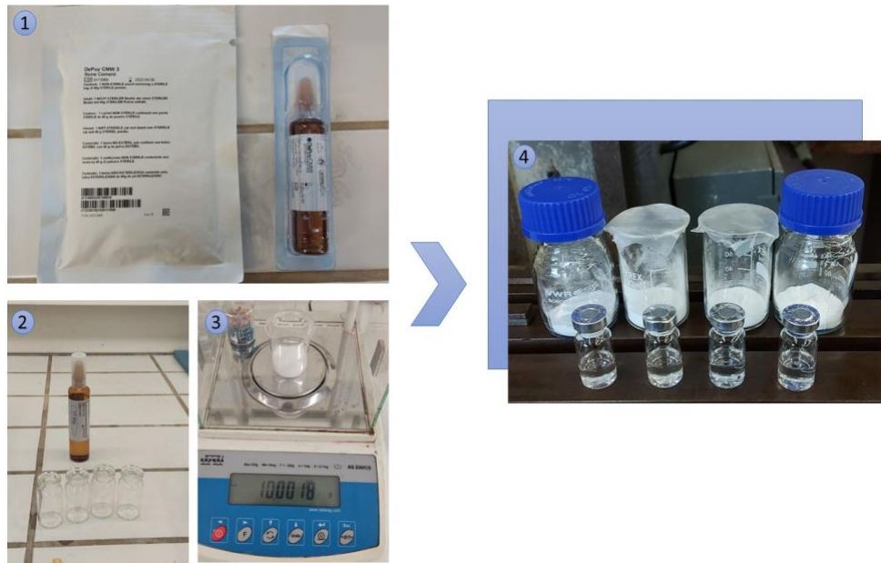
Fig. 2 Bone-Cement production process.
