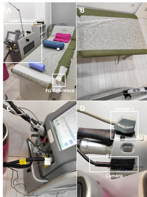
Figure 2. Laser treatment room. The laser device is located to the left of the surgical bed (A,B). On the handheld laser device, the electromagnetic sensor and a camera were attached (C,D). Note that FG refers to field generator.
