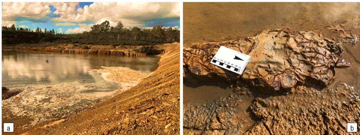
Fig. 2. Accumulation of ochre precipitates (a) with colloidal properties along channel bed (b).
