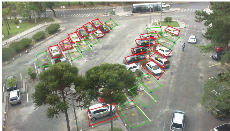
Figure 1: An example of the identification of the availability of parking spaces in open parking lots using DL [10]. The green and red rectangles show the availability and unavailability of parking spaces
