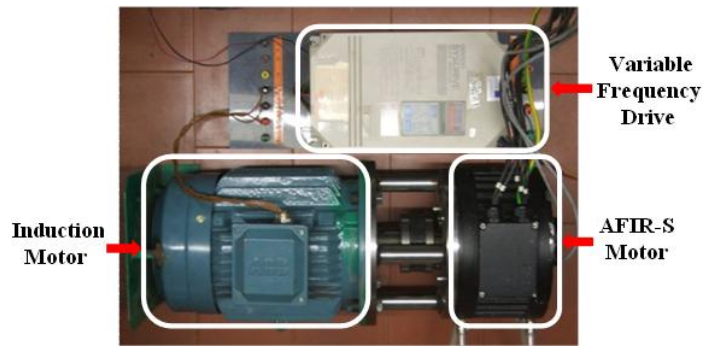
Fig. 7. Test bench assembled to synchronize the AFIR-S windings.
