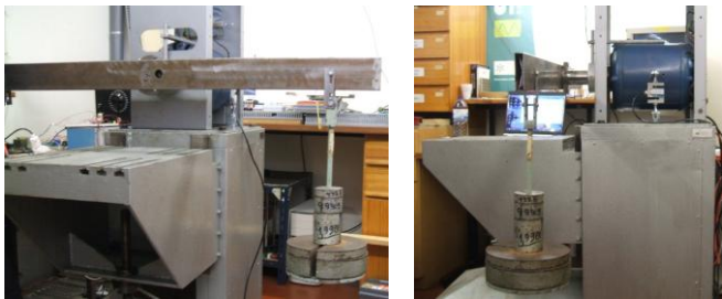
Figure 9. Calibration process of load cell with weights.
