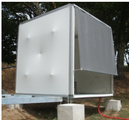
Fig. 41 – Membrane test Cell at the University of Minho, Portugal (Mendonça, 2010).
