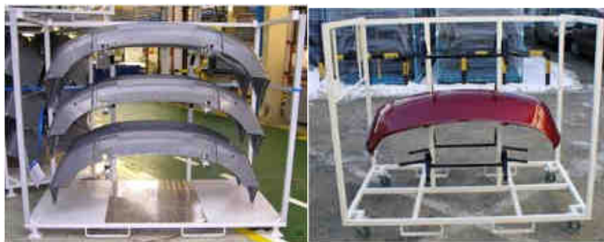
Figure 140 – Transportation units for coloured bumpers
